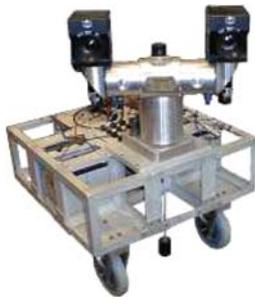
Figure 1. The Yorick stereo pan-tilt head (Sharkey et al., 1993), and robot GTI, used for visual navigation.
